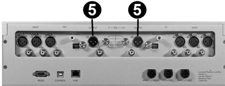
The inner XLR connections on the rear of the Perseus are outputs. To remove an XLR plug, push on the tab on the connector body and pull the plug out. Be sure to match the output to the correct channel on your preamp. As you are looking at the back of the Perseus, the output on the left side is for the right channel, the output on the right is for the left channel.
